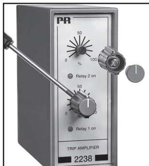
Picture 2: Removal of knobs.
